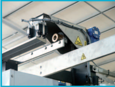
DETAIL OF DOORS MOVEMENT
